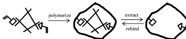
FIGURE 1. Highly schematic representation of the strategy of molecular imprinting.
